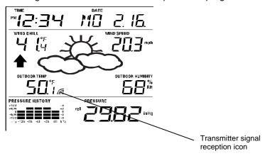
• If the signal reception is not successful on the first frequency (915MHz) for 45 seconds, the frequency is changed to 920MHz and the learning is tried another 45 seconds. If still not successful, the reception is tried for 45 seconds on 910MHz. This will also be done for re-synchronization.
